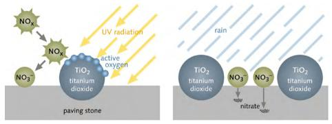
Fig. 7. Reaction process - How TioCem reduces NO,
