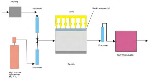
Fig. 4. Scheme of testing equipment for  $NO_x$  as in standard 11247:2007
