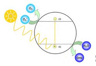
Fig. 1. The principle of formation of hydroxyl radicals OH-
